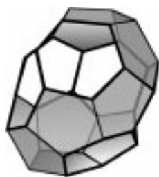
Figure 4. Model of the larger and unsymmetric cage in Sigma-2. The cage is composed of 5- and 6-rings and contains the adamantamine molecule. A comparison with Figure 1 suggests that the large cavity in SSZ-25 is more than twice as large. One question that arises is whether there are two adamantamines per large cavity in the synthesis with this template.
